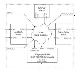
Fig. 4. MiCAP with single port RAM.
