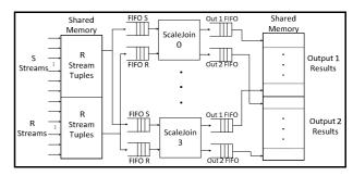
Fig. 3. FPGA-based ScaleJoin architecture
