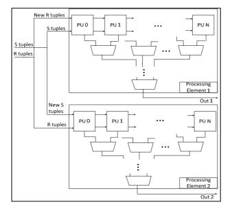
Fig. 2. Reconfigurable StreamJoin architecture
