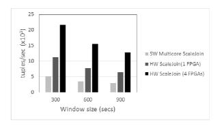
Fig. 5. Throughput (tuples/sec) for SW-based multicore ScaleJoin and FPGA-based solution ScaleJoin
