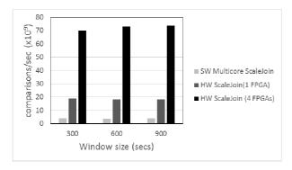
Fig. 4. Processing rate (comparisons/sec) for SW-based multicore ScaleJoin and FPGA-based solution ScaleJoin
